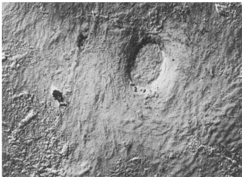
FIGURE 5 The lumen wall of a white oak fiber tracheid on the veneer surface after a hot-water extraction, showing most of extractives were removed but some resisted the solvent extraction (3,4000 \times ).
